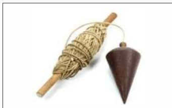
LINE DORI WITH PLUMB
