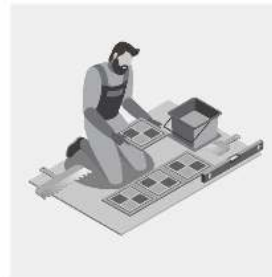
Step-3 Laying of tiles on the Surface
