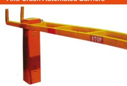
Fixed Length 4m/4.5m **Heavy Duty AC Motor** Double Side Mild Steel, Heavy Duty Boom Boom approx-30-50Kg with counter balance 2 buttons to control the barrier gate. Operation time 7-8sec depending on length of the boom Technical Specs: 220 V AC +/- 13% / 50Hz / 120 Watts. Control PCB Operation : Manual/Remote Control/ Push Button Optional Operation :Rfid/ NFC/Biometric/Loop Detector Third party Access control
