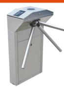
Turnstiles are compact and cost-effective entrance solutions Designed for Low Traffic Volume . Capacity: 15-25 /min, AC110-220V,50Hz/60Hz, Power Consumption :60w Alloy steel tripod hub prevents mechanical wear Casework and tripod arms manufactured in SUS304 stainless steel
