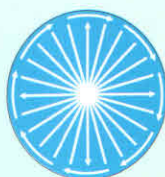
0° lead Average material will be thrown straight
