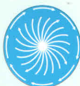
30° lead Average material will begin to spiral
