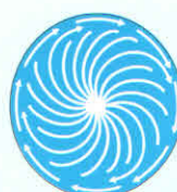
60° lead Average material will give maximum screening pattern
