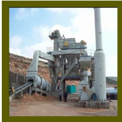
Asphalt Batch Mix Plant 80tph
