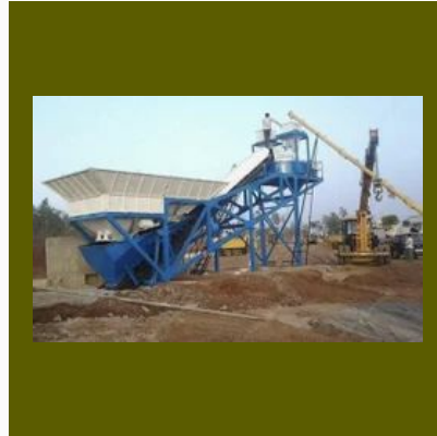
Concrete Batch Mix Plant
