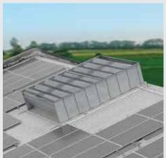
Low Profile design allows this sheet metal ventilator to sit just 940 mm above the roof line. It is designed for a wind velocity of 50 m/sec (180 kmph) which exerts a pressure of 2.039 kN/m2 on the vertical face. The resultant maximum support reactions at the any mounting point are restricted to
