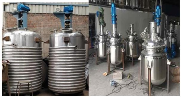
Reactor is mostly known as Chemical Reactor, Industrial Reactor, Jacketed Reactor, Limpeted Reactor, Pharmaceutical Reactor, Process Reactor, Stainless steel Reactor, Agitated Reactor, Mixing Vessels etc
