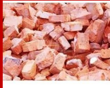
Brickbats for Waterproofing
