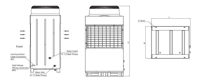
Storage tank: Minimum 2000 & 4000 litre for 5HP & 10HP respectively Circulation pump flow rate: 3500 LPH & 6500 LPH for 5HP & 10HP respectively Recommended water hardness: Less than 300 ppm
